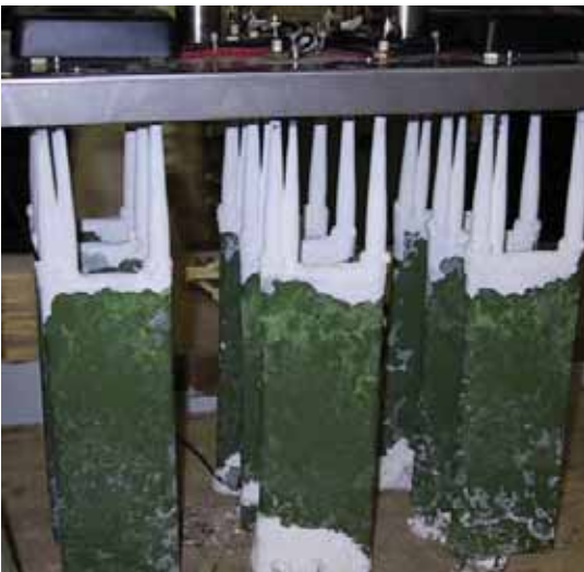
Teflon-coated heaters after 720 operating hours with water at 28 °F hardness (500 µS/cm). No manual cleaning has been performed. The layer of Teflon® assists the spontaneous separation of the lime scale, while the excellent heat conduction of the aluminium alloy avoids any localised overheating.
